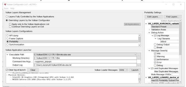
This configuration includes the Khronos Validation Layer and the Device Simulation layer. To the right, we can see the layer settings.
