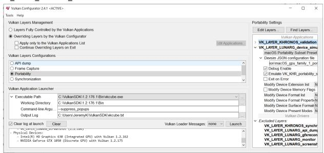
Now, copy-paste the path of your config file into the "Devsim JSON configuration file" textbox and uncheck the "Emulate VK\_KHR\_portability\_subset" option.
